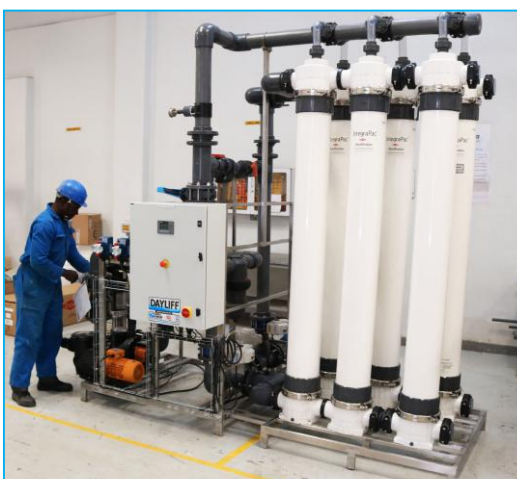
A Dayliff Ultrafiltration plant (DUF) under production at D&S HO Technical Division in Nairobi.
