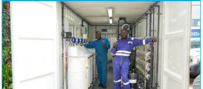
D&S South Sudan under Manager Lodu Gabriel have supplied a containerised water treatment system with Dayliff Ultrafiltration (DUF) and Reverse Osmosis (DRO) technology to a large oil and gas client. The mobile system will produce totally pure and safe water wherever it is deployed. Pictured are D&S technicians Sylvester Omondi and William Osala during the commissioning.
